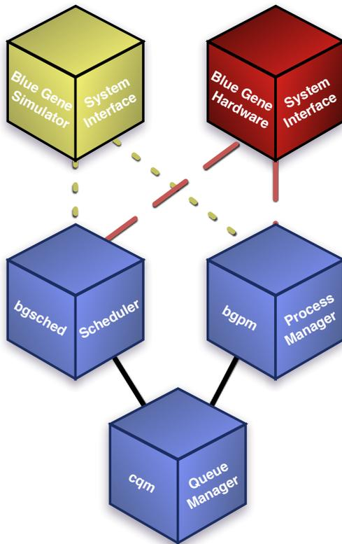
Fig. 2. Blue Gene/L Simulator Architecture
